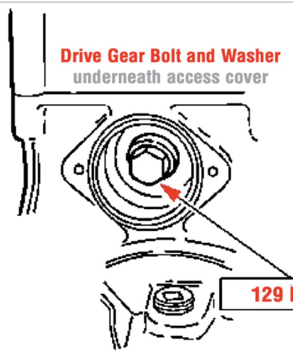
**Drive Gear Bolt and Washer underneath access cover**
