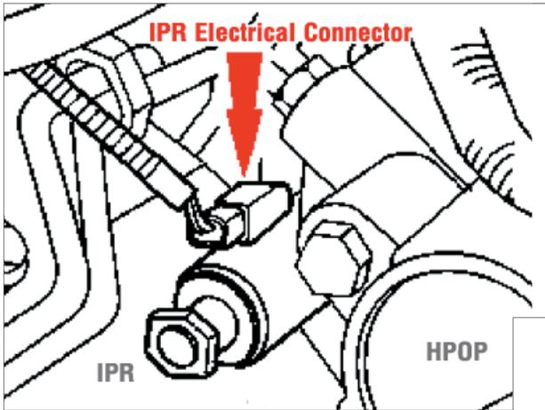
Disconnect the electrical connector from the injector pressure regulator.
