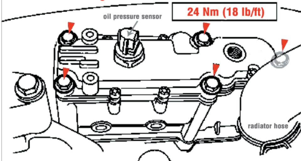
Remove the (3) 10mm bolts and (2) 13mm bolts holding down the reservoir. Remove the reservoir with the fuel bowl attached.
