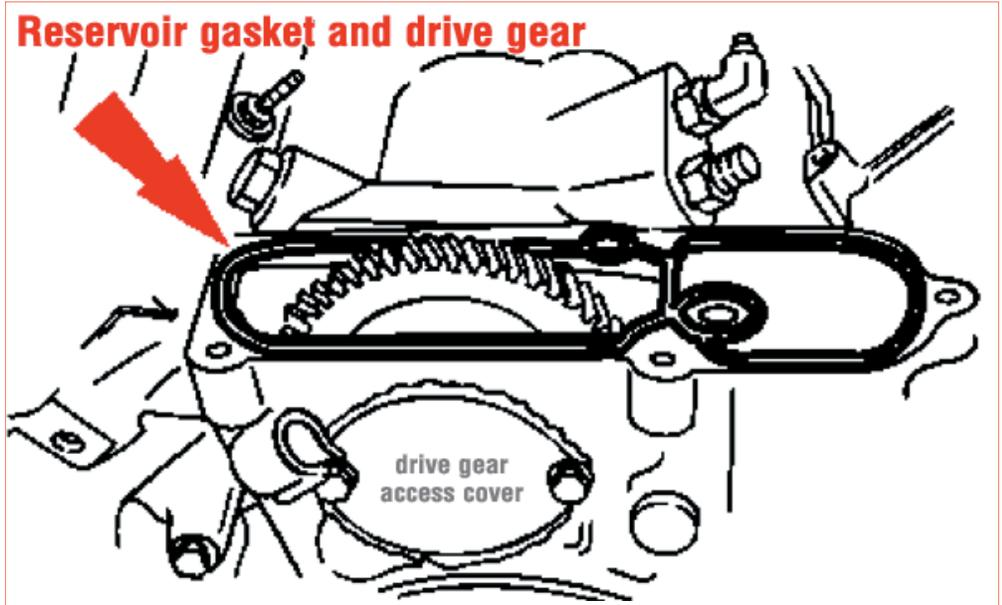
**CAUTION:** Make sure that the drive gear is fully seated on the high-pressure oil pump before installing the bolt and washer. Otherwise, the drive gear may not seat properly, causing binding or slippage resulting in a no oil flow condition. Do not assume the bolt will pull it tight and flush.
