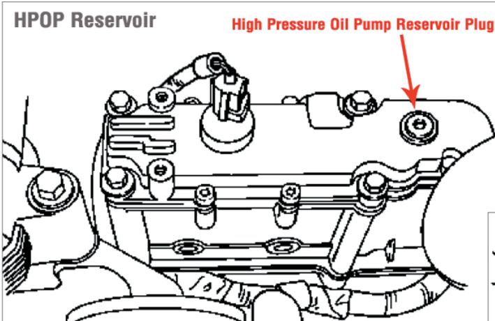
Remove the high-pressure oil pump reservoir plug using a 3/16" allen wrench. Using an oil suction device, remove the oil from the high-pressure oil pump reservoir. If you do not remove the oil before removing the reservoir, it will not harm anything. However, it will make a mess as you will dump about 3/4 quart of oil all over your engine.
